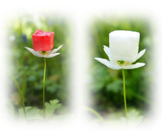
Figure 1: Polysaccharide aerogels: highly porous and light-weight materials.
