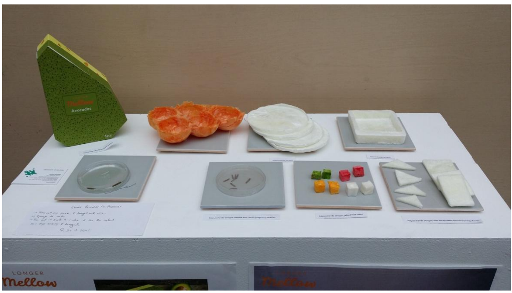
Figure 3: PackAge student project (Polysaccharide aerogels: future active food packaging concept) and other aerogel samples displayed at Designing Cellulose for Future exhibition.
