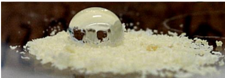
Figure 1. Water droplet on hydrophobic NFC grafted with poly(ethyl acrylate) (NFC-g-PEA).
