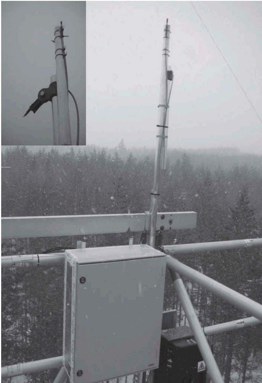
Figure 1. The spectrometer system is mounted on a metal rod at the top of a scaffolding tower. The target-looking fibre can be slid up or down and rotated around the rod to change the measurement footprint size and location.
