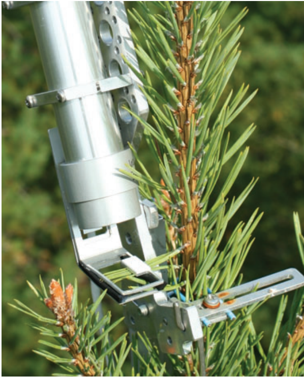
Fig. 1. A MONI -head measuring ChlF from Scots pine needles in a top canopy shoot. With the help of the custom-made supports, MONI -head and needles remain in exactly the same position relative to each other throughout the year.
