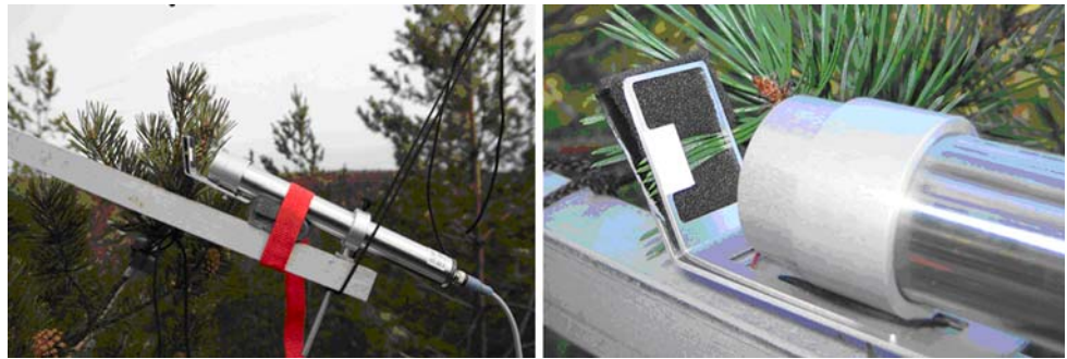
Fig. 1 MONI -head emitter-detector unit in a semi-permanent installation at the top of a crown of Scots pine (left), and details of the sample holder with Scots pine needles (right)
