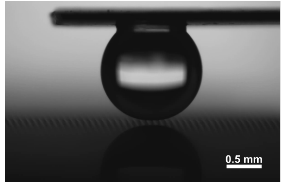
Figure 1: SDAM droplet probe in contact with a superhydrophobic micropillar array surface.
